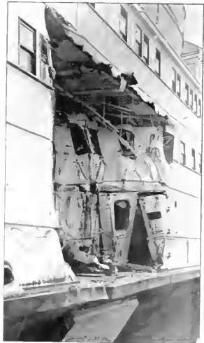
At the left we have the bow of the American tanker Swift Arrow on the dock at the Robins plant of Todd Shipyard Corporation after her collision with the steamship Boston on July 21. At the right is shown the steamship Boston after this collision while undergoing repairs at the Tietjen & Lang plant of the Todd Shipyard Corporation. A feature of this collision was that all the casualties were due to the crushing of passengers in their staterooms. No access was possible to the victims until after the vessel had been towed to port. Had the vessel been equipped with portable oxyacetylene cutting apparatus immediate aid might have been rendered, some lives might have been saved, and certainly much suffering could have been avoided.
